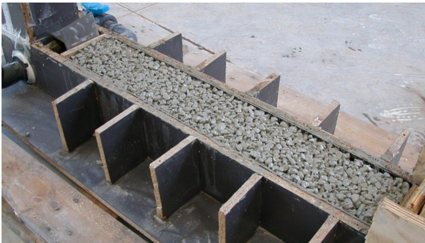
Figure 1. Pervious concrete inside permeameter of laboratory
