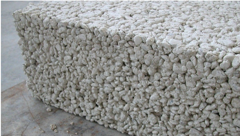
Figure 7. Photocatalytic pervious concrete slab
